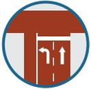
Installing turn lanes extend required pedestrian crossing times. Bulb outs or median refuge islands may be considered in these locations to help shorten the required pedestrian crossing distances.
