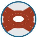
Roundabouts or alternative intersection layouts may be considered in certain situations to help resolve skewed approaches, particularly if multiple legs of the intersection approach at odd angles.
