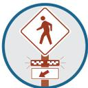
RRFBs may be located on each side of the road or on both sides for a single direction travel lane. The signs may be solar powered in rural areas. Best practice includes RRFB signage on each side of the roadway and in the center median for both directions of travel, when feasible.
