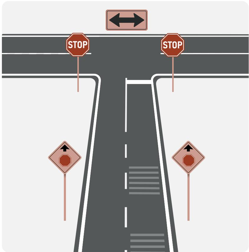
A combination of several low-cost safety countermeasures may be installed to improve safety at unsignalized intersections. Countermeasures may include installing turn lanes, upgraded signage, and improved striping. Intersection lighting and rumble strips may also be incorporated.
