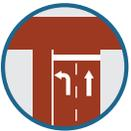
Ensure sight distances are maintained with the addition of signage, turn lanes, or lighting. For lighting to be included in low-cost measures the availability of power needs to be evaluated.
