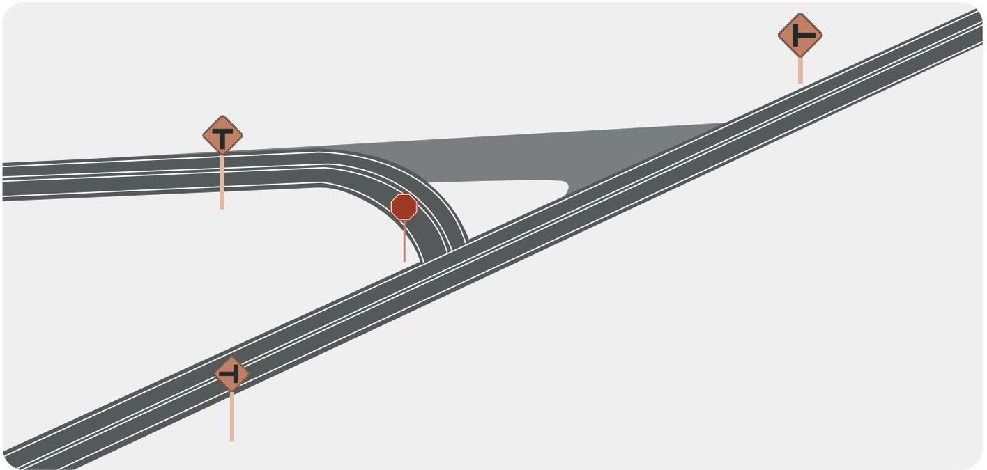
A misaligned or skewed roadway approach (typically a more minor local or collector type roadway to a larger collector or arterial type roadway) creates sight issues for motorists and increases crash risk to all roadway users, including pedestrians and bicyclists. Realignment countermeasures including repaving, striping, signage, and roadway configurations provide better sight distance and visibility at the intersection for all users.
