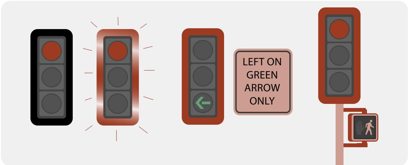
Various safety countermeasures may be applied at signalized intersections. Countermeasures may include signal timing adjustments, signal infrastructure components such as signal heads or lighting, and lane geometries at the intersection.
