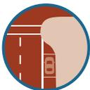
On-street parking must be restricted approaching bulb outs as to not block visibility of pedestrians to motorists. Bulb outs should not extend into the travel lanes. Bicycle lanes need to be considered in the roadway cross section, particularly at the bulb out locations. Drainage should also be considered, especially if bulb outs are extending or covering curb and gutter.
